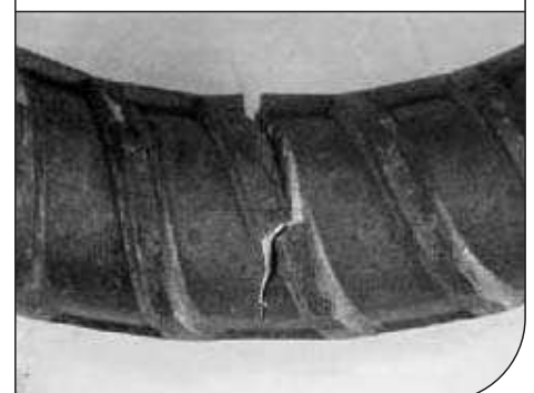
Figure 2 Cracks in Grade 500 reinforcement caused by incorrect bending and rebending
